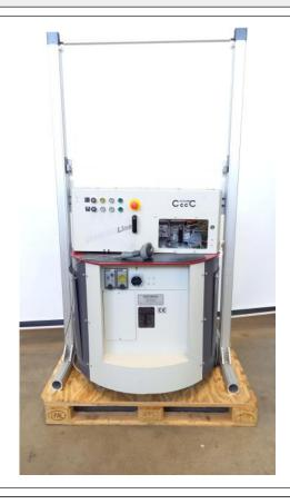
The FourC machine is for automatic measuring of gemstones which are not undercut during the rotation.
